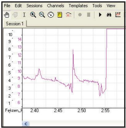
TEST OF STOCK INJECTORS TO THE LEFT AND M3 E36 INJECTORS TO THE RIGHT, MADE IN THE SAME CAR ONLY WITH DIFFERENT SOFTWARE.
